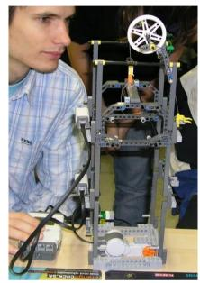
Figure 4. A lift using light signals
